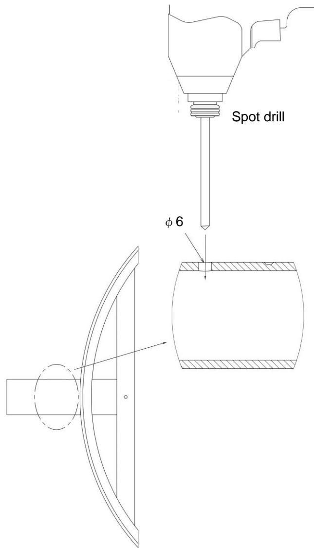
Ensure that no swarf enters inside the clock while drilling a hole.
