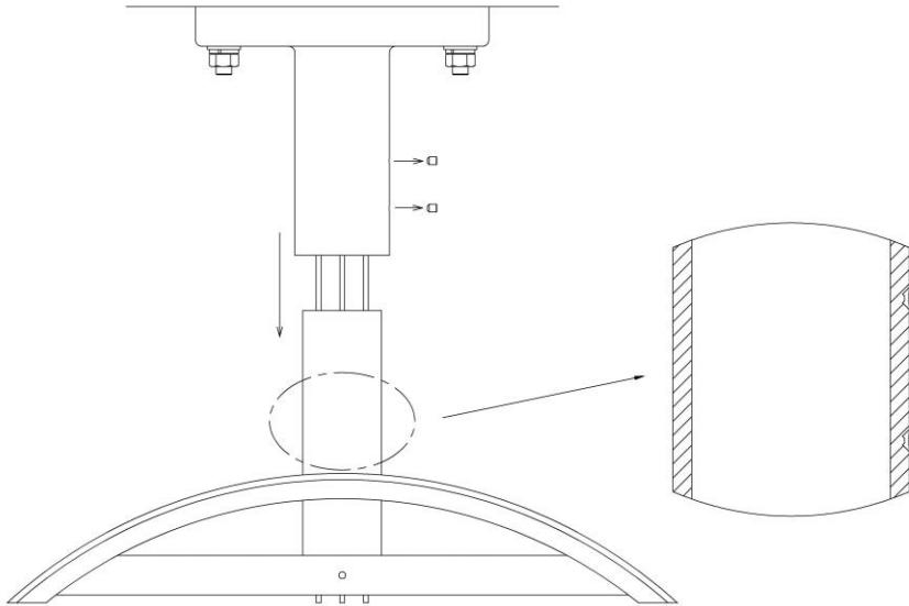
While loosening the screws, be sure to have another person hold the clock. If this step is performed by only one person, the clock may drop to the floor.
