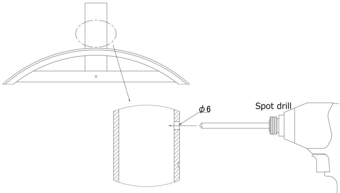
Ensure that no swarf enters inside the clock while drilling a hole.
