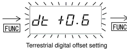
With each press of **+** or **-**, the time correction setting display changes in the following or reverse order, respectively:
