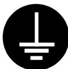
Connection of grounding conductor
